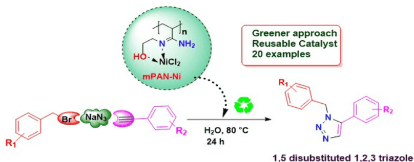
Scheme 1: Schematic representation of AAC using mPAN-Ni
